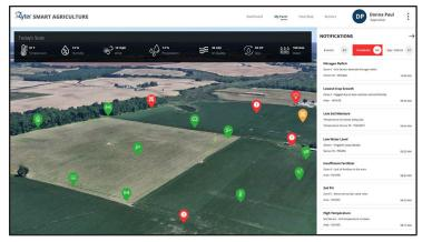
Receive instant alerts if any important parameters that are being monitored drift out of pre-set ranges.
